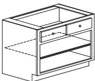
Any base cabinet may be ordered without doors, drawers remain. Finished interior to match exterior. One full depth adjustable shelf 3/4" solid wood.
