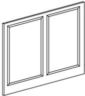
3/4" thick solid wood panels used to finish backs of cabinets. Both ends and top edges are finished. Each wainscot must indicate if it is to be manufactured with integral panels or applied non-operational doors. Maximum length - 96".
