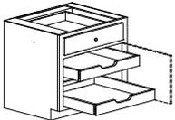
5/8" Solid wood pull out trays may be ordered for any cabinet. Specify location and number. If one tray is ordered it is fixed and on the bottom of the cabinet. If more than one tray is ordered, all are adjustable.
