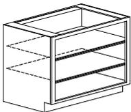
Any base cabinet may be ordered without doors and drawers, finished interior to match exterior. Shelves are adjustable, full depth and 3/4" thick.
