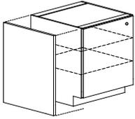
A 3/4" thick pilaster may be added to the end of any frameless base cabinet. The pilaster will be flush with the top, bottom, and back of cabinet, and will protrude beyond cabinet face to line up with the front of cabinet door. The cabinet width will increase by 3/4" for each pilaster added.
