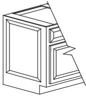
Integral inlay panel manufactured into the side of a base cabinet. Overall width of cabinet does not change.
