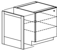
A 3/4" thick door pilaster may be added to the end of any frameless base cabinet. The pilaster will be flush with the top, bottom, and back of cabinet, and will protrude beyond cabinet face to line up with the front of cabinet door. The cabinet width will increase by 3/4" for each pilaster added.
