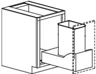
Large 50-quart plastic container installed in a solid wood framed box 8" high. 150 lb. soft close drawer slides. Door is attached to wood box. Metallic Silver Polymer wastebasket. Unit fits in BX 18.
