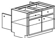
Face frame and doors on both sides of cabinet. Drawers operate from front side, false panels on back. BX cabinets will have full height doors both sides. Cabinet depth does not change.
