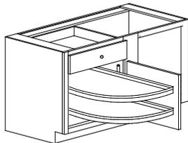
Swing out shelf constructed of 5/8" plywood with a vinyl band with a 1" high edge. Recommended for BC 42, 45 and 48 only.
