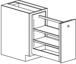
Door attached to a wood insert with full extension slides. Insert has one fixed drawer box on the bottom, and two adjustable shelves above.
